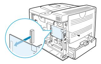
5 Align the connector on the network or serial interface card with the connector on the control board. Push the card firmly into the connector until it is completely inserted into place.
